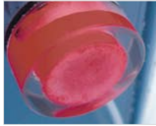
Corrosion-protected electrode junctions
